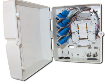
distribution and dispatch of finer inn nodes between feeder cable and branch fiber cable. The maximum capacity for this box is 36 fibers, it can be installed 4x1: 8 PLC splitters. It is especially suitable for building network construcion with application of PON technology.
